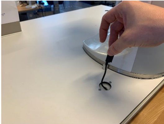
Figure 2–63: Pulling the ARS cable
