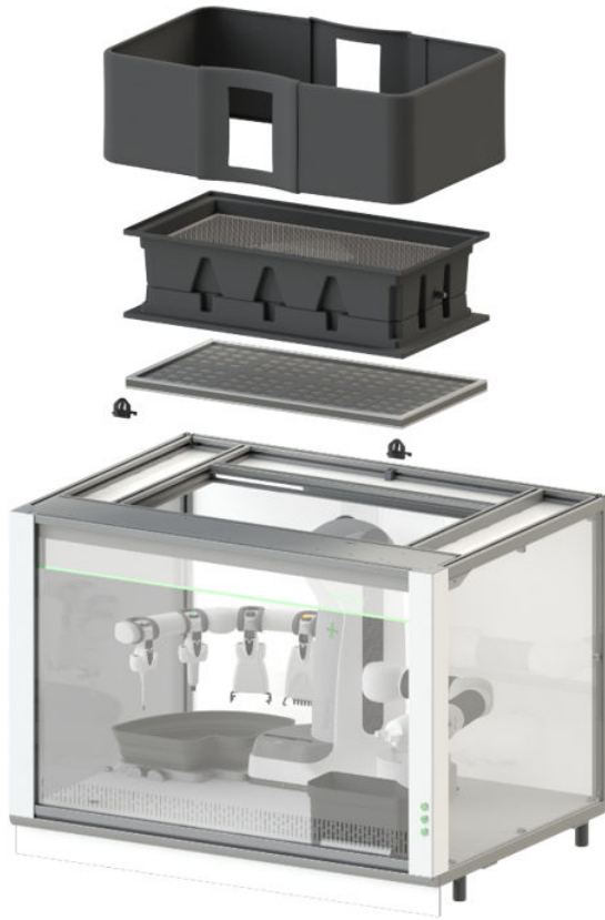
Figure 2–29: Ventilation module without filtration configuration
