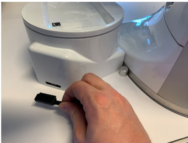
Figure 2–65: Connecting the magnetic connector to ARS
