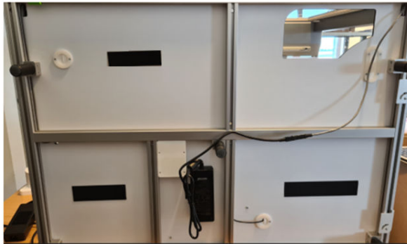
Figure 2–11: Installing the external power supply
