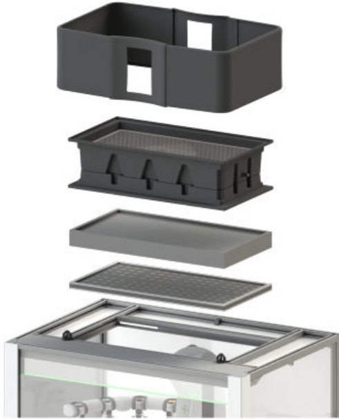
Figure 2–40: Filtration fume cabinet configuration
