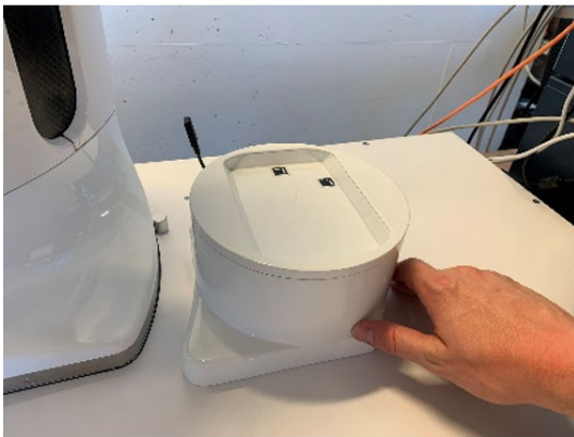
Figure 2–64: Placing the ARS unit
