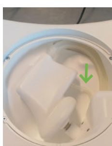
Push the small hose to straighten it
