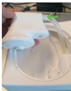
Take a new filter, and plug in the big hose first
