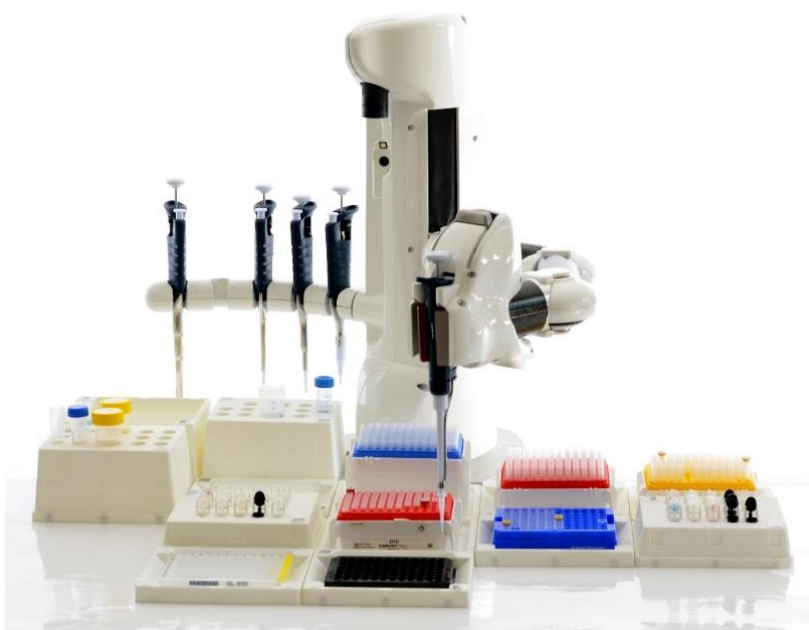
FIGURE 2. ANDREW, THE PIPETTING ROBOT USING MANUAL PIPETTES.
